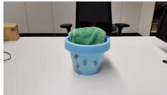
(b) Cup with markers that are used for tracking its position. At least 4 markers are needed to create a rigid body in OptiTrack.
